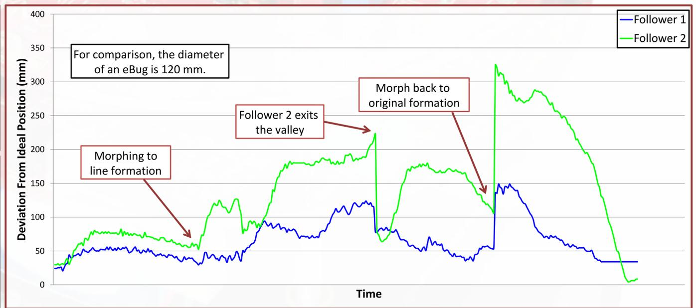
Results show that the followers are on average 101 mm away from the ideal position, which is less than the diameter of an eBug. It also demonstrates that the eBugs are able to navigate through environments with obstacles without any collisions.
